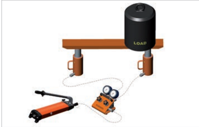
→ Asymmetric load: Recommended total cylinder capacity = 2 x load
