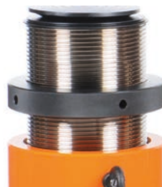
Multiple-start and rounded thread on plunger for a quicker positioning of the locknut and easy dirt removal
