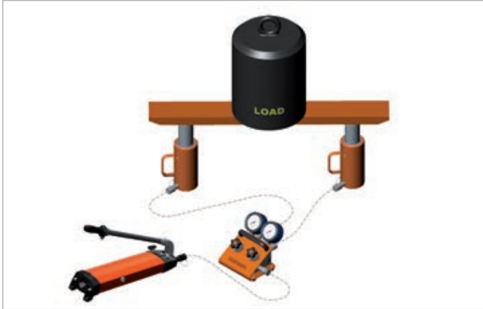
→ Symmetric load: Recommended total cylinder capacity = 1.5 x load
