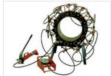
A complete set-up in which a cylinder has been placed on every bolt (so-called 100% occupation)
